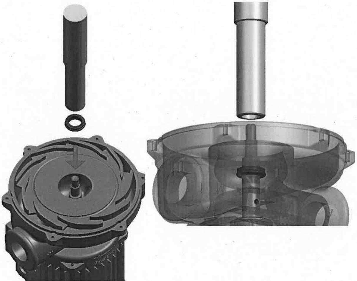
6B) Assemble the movable part of the mechanical seal using a pair of pliers.
